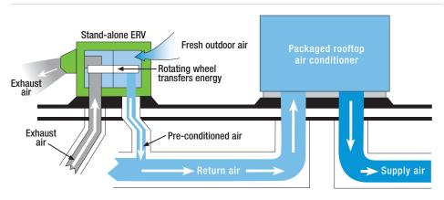
A stand-alone ERV system is installed near your existing air-conditioning unit. It is capable of removing air from spaces such as offices, breakrooms and restrooms that needs to be removed anyway.
